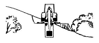
Dig field trenched progressively. As soon as one trench is completed, have the workmen lay the tile. Start the next trench, using the spoil to fill the previous trench.
